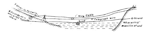
The traveller was an ordinary pulley block in this case. The boat here was provided with 2 tow ropes, the advantage being that the standing end of the one not in use could be undone and sent across while the boat was in transit, thus giving more time for the operation which took a little time owing to the width of the river and force of the current.
